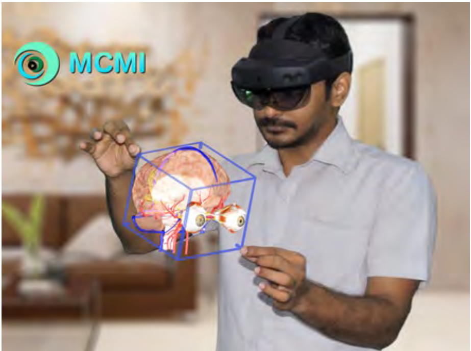
Figure 1: The user is wearing the head-mounted HoloLens 2 device to experience the extended reality (XR) 3D holograms.
